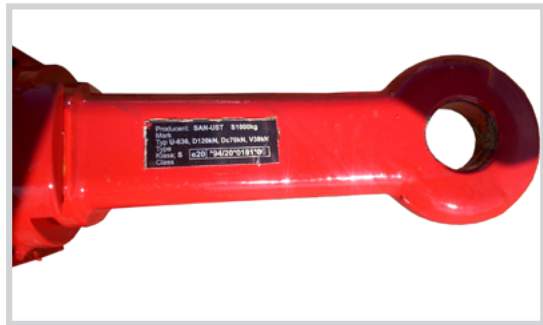
Ø40 mm automatic ring hitch
